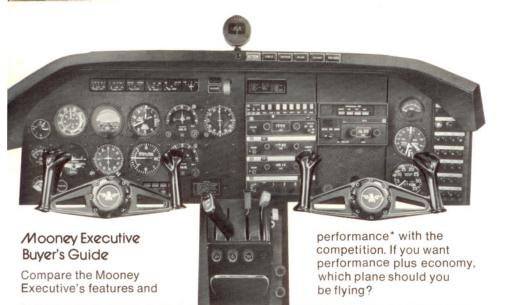
A pro's panel. Arranged the way panels should be for those tough IFR flights, including T-grouped flight instruments (standard), professional annunciator light stack, room for complete primary and backup avionics. Choice of Narco or King packages clean-room tested and factory-installed for reliability.
